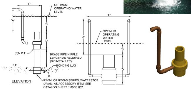
SPECIFICATION DATA: Bubbler Nozzle; cast bronze construction, copper venturi air intake snorkel and (F) N.P.T. threaded connections. (Optional alignment swivel available as an accessory item; see catalog sheet 1.802).
