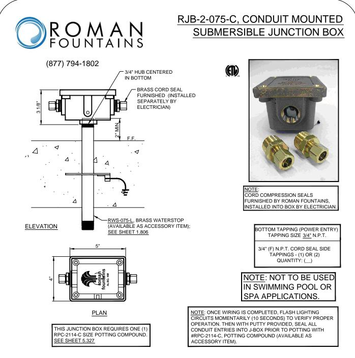
SPECIFICATION DATA: ETL Listed Conduit-Mounted Submersible Junction Box, cast bronze construction, with neoprene gasket, stainless steel fasteners, (1) 3/4" (F) N.P.T. bottom power conduit connection, and (\_) 3/4" N.P.T. side connection with brass cord seal fitting (shipped loose and installed in field). Junction box shall have a minimum volume of 20.0 cubic inches and shall include an internal grounding lug.
