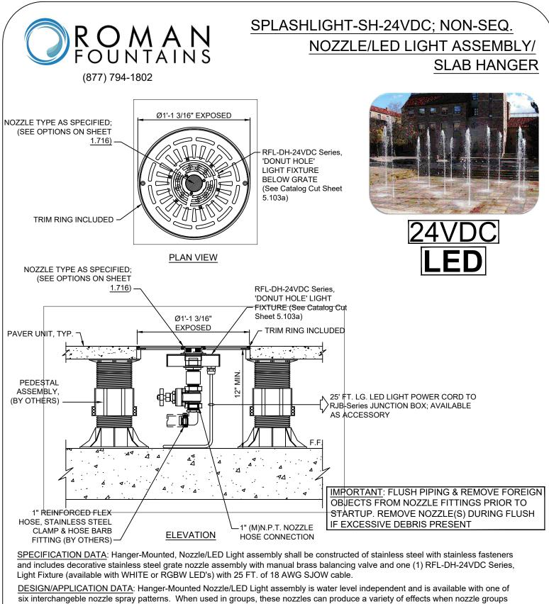
six interchangeble nozzle spray patterns. When used in groups, these nozzles can produce a variety of effects when nozzle groups are piped below deck in various patterns and switched on and off via sequenced controller and remote solenoid valves (both items are available as accessories). The nozzle groups can also produce varying stream heights when used in conjunction with a sequenced variable speed pump drive (VFD's also available as an accessories).
